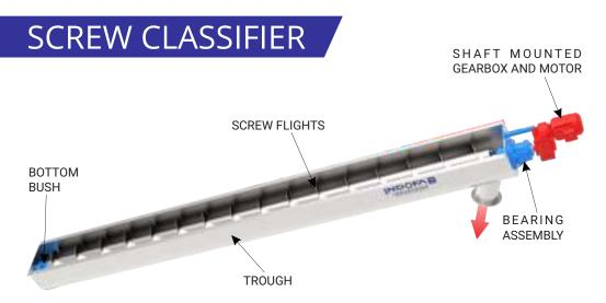
This type of Classifier consists of slow speed Single Screw enclosed in a half metal trough for positive material transfer ensuring higher rate of grit/sand disposal. Screw Diameter, length and angle of installation can be more flexibly designed to suit the application
