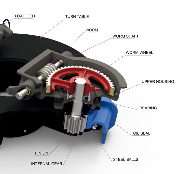
• The above entire system together with a suitable Gear box & Motor is termed as Centre Mechanism or Pier mounted Drive.
